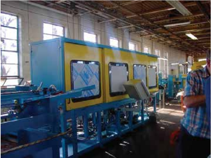
Finishing up a Vulcan Ultimate with a sound enclosure.
