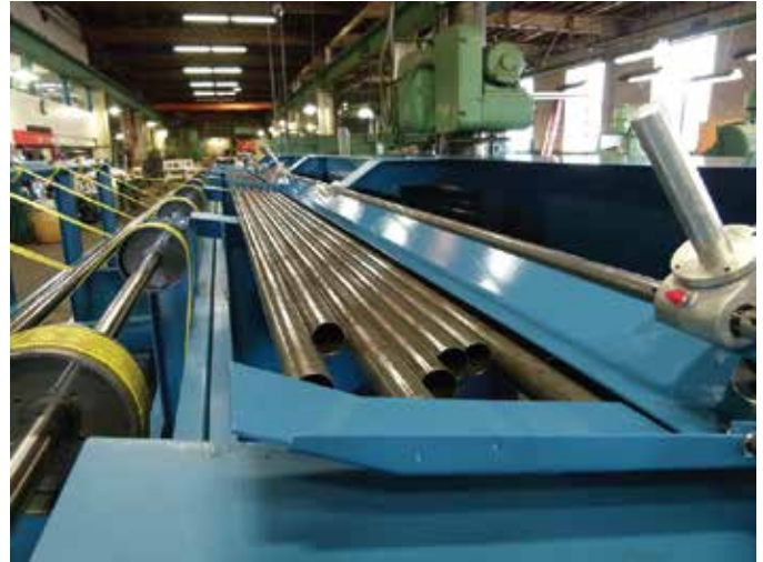
Tubes being loaded for high-speed cutting process.
